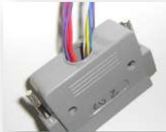
Wires can vibrate within the connector housing
