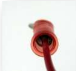
Wires can vibrate near the connector
