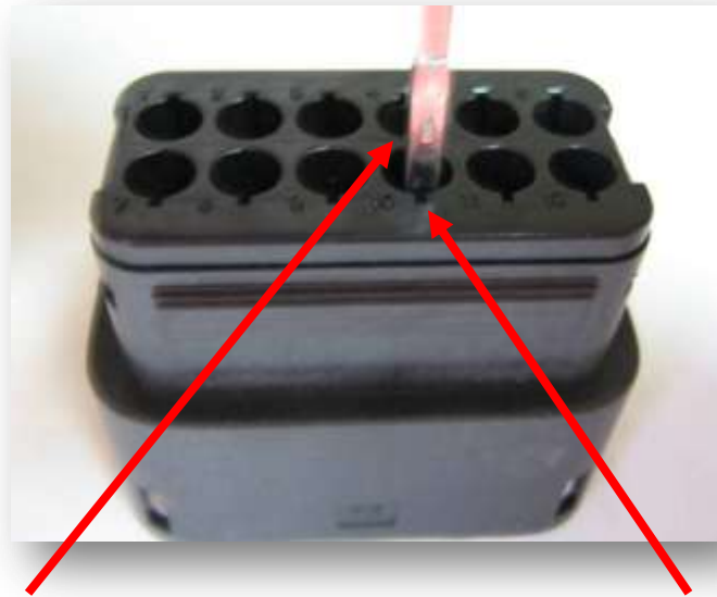
Orientation feature aligned with index
