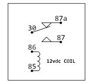
NORMALLY CLOSED CONTACTS (30 to 87a) RATED AT 20 amps
