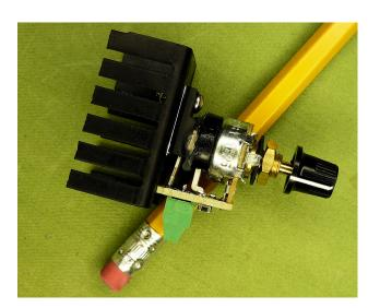
o dim the interior lights or instrument panel lights of the certificated aircraft you trained in, you turned a knob attached to an Ohmite Series-A wirewound rheostat. Somewhere behind the Royalite was a smoking hunk of ceramic wound with toaster wire. A finger holding a chiclet of graphite picked off the desired voltage. The whole thing weighed easily as much as a cheeseburger.
