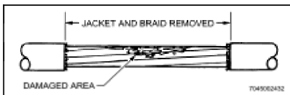
Figure 5-18 Damaged Multi-conductor Cable
