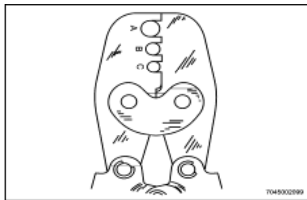
Figure 10-61 AMP 220066-1 Ferrule Crimping Tool Showing the Three Crimping Dies
