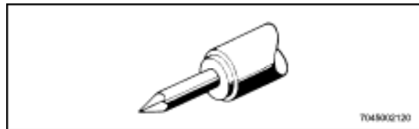
Figure 12-14 Correct Shape for Soldering Iron Tip
