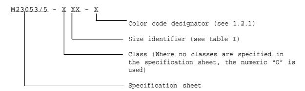
Example: Class 1, gray (slate), 0.250 inch (6.35 mm) as supplied ID sleeving shall be identified as M23053/5-106-8.
