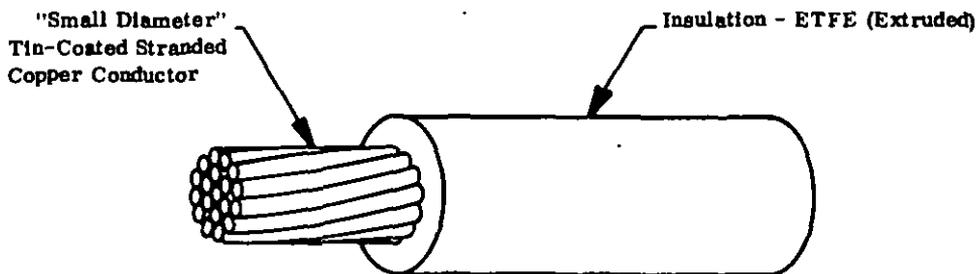
ETFE - Ethylene-Tetrafluoroethylene Copolymer
