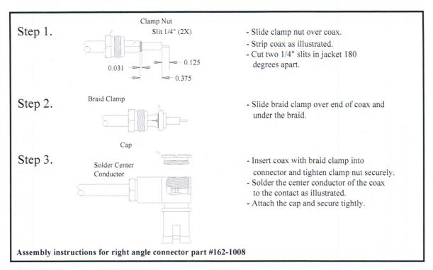
Figure 4 Coax Connector Assembly
